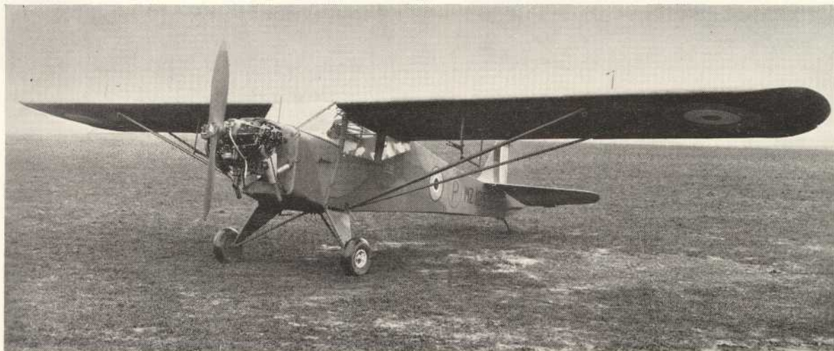
The prototype AUSTER Mk. 2. Due to the short supply of Lycoming engines at that time, the Mk. 2 was abandoned in favour of the Mk. 3, which was fitted with the more readily available DH Gypsy Major 1 engine.
