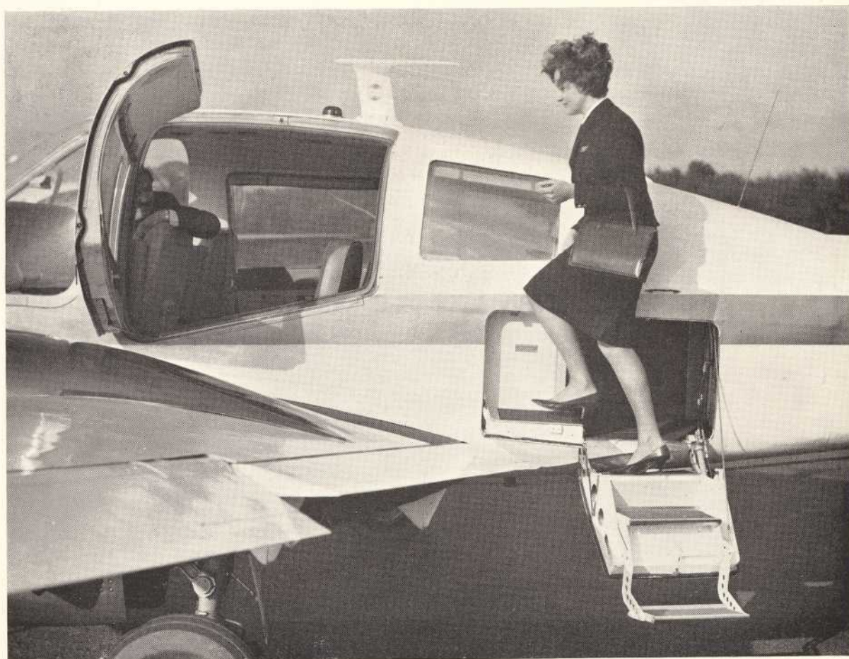
STEP ABOARD the Beagle B.206 – ease of entry is ensured by the provision of a wide 'limousine type' door (46 in. x 36 in. high) together with the hydraulically operated 'air-stairs'.
