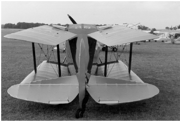
A modern photograph of G-ADLY with wings folded. This feature enabled more storage solutions.
